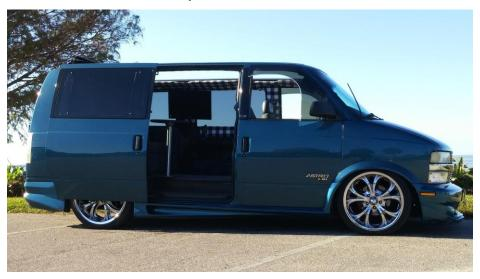
The van began its days as a V6 passenger van and now the van has a 1998 LS1 engine paired with the 4L60e automatic transmission. All the power goes to a custom 4 link Ford 9" rear with 3.56 gearing. The van has an air ride suspension with front and rear Firestone bags, two Viair compressors and three 5 gallon air tanks. Each wheel has its own control valve and is controlled by a Dakota air management system.
