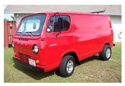
Red Ryder is a 1966 GMC Handi Van with a 307 V8 and a turbo 350 transmission it has 373 gears in the rear end I have completely gone through
